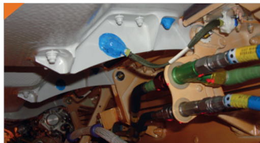
FIG 1: ELECTRICAL BONDING POINT ENCAPSULATED IN NYCOTE 7-11 BLUE
